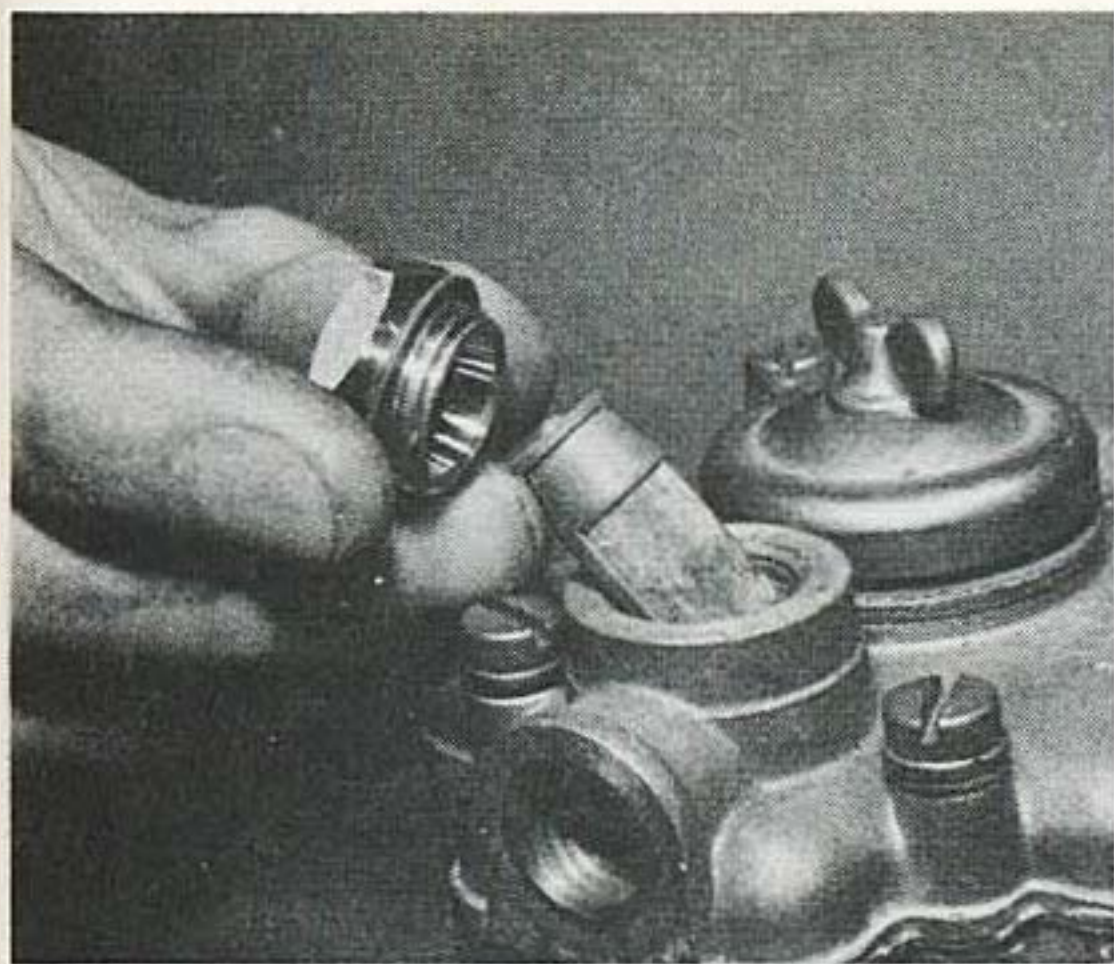
5.2 Removing the fuel filter
