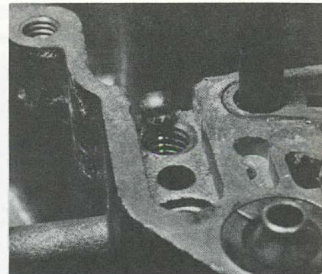
7.30 Fitting an accelerator pump delivery valve ball
