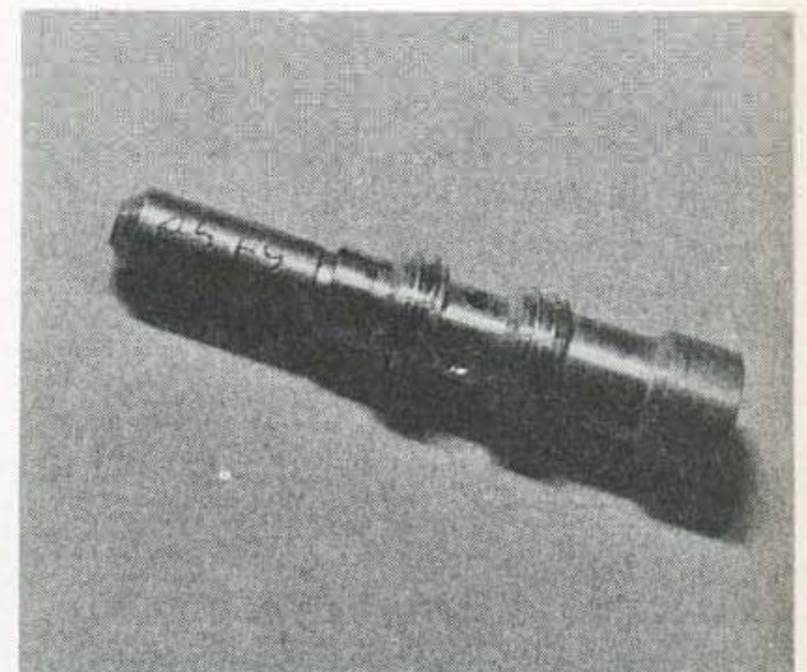
5.12b Idling jet sections assembled
