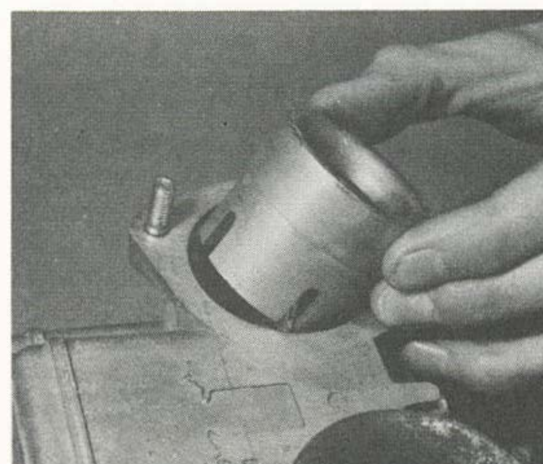
5.38 Removing a choke from the carburetor barrel
