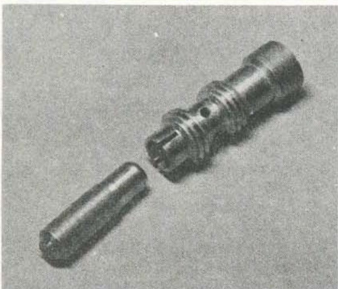
5.12c Idling jet components
