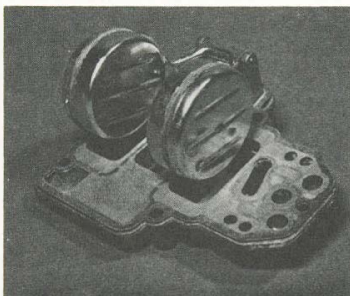
7.40 Gasket and float assembly fitted on the carburetor cover
